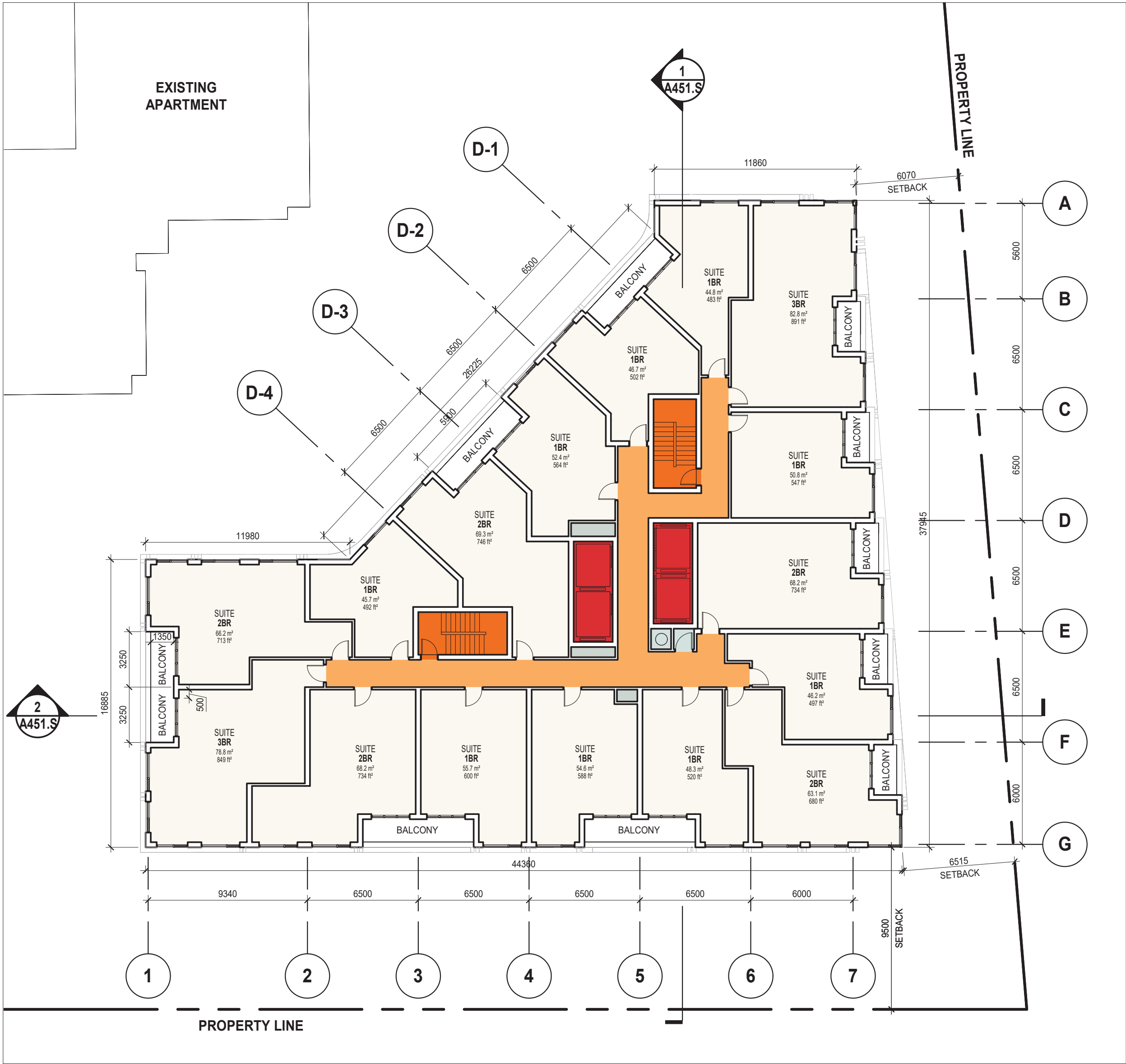
2 A202.S TYPICAL PODIUM FLOOR PLAN -2ND TO 4TH LEVEL
